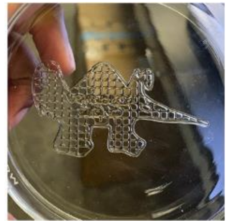
UCI mascot (Peter the Anteater) generated during student training course on 3D bioprinter
